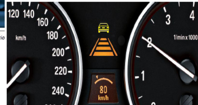
Figure 25. Head down display with ACC symbol showing system is active, user set distance as number of visible orange bars and cruise speed set to 80 km/h. Source BMW
